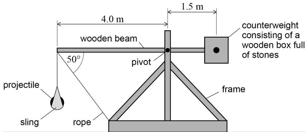
The counterweight is a wooden box full of stones attached to one end of the beam. The projectile, usually a large rock, is in a sling hanging vertically from the other end of the beam. The weight of the sling is negligible. The beam is held horizontal by a rope attached to the frame.
